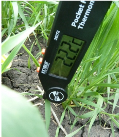
Figure 18. Temperature at 5 and 10 cm using a pocket thermometer (left) and at the surface using the Apogee IR sensor (right)
