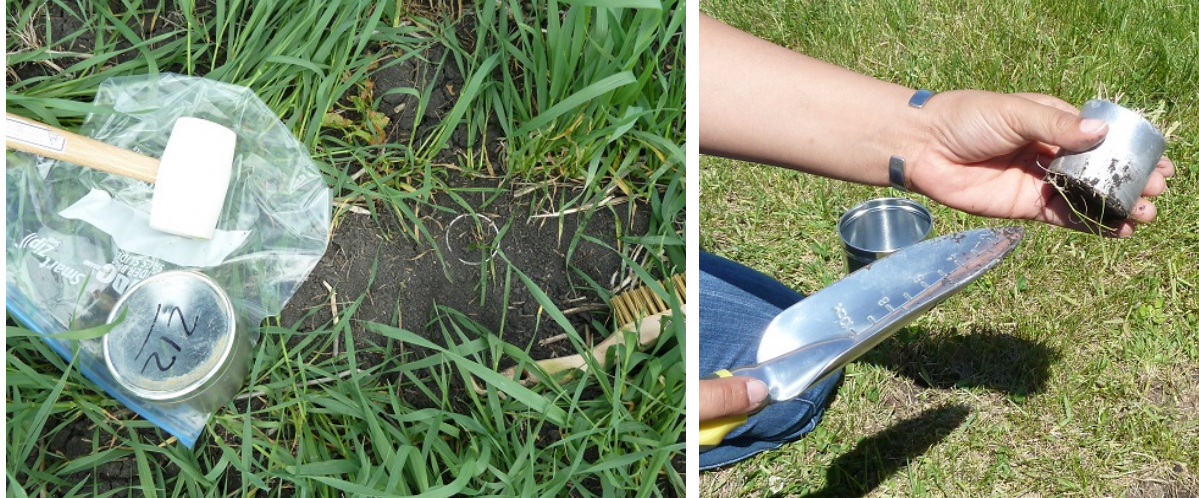
Figure 17. Soil core in the ground (left) and following removal (right)
