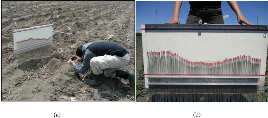
Figure 19. Measuring surface roughness using the pin profiler
