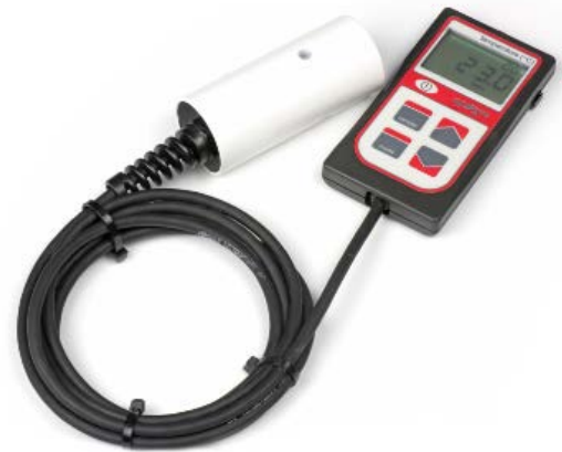
Figure 18. Temperature at 5 and 10 cm using a pocket thermometer (left) and at the surface using the Apogee IR sensor (right)
